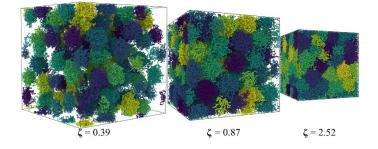
Representative snapshots of neutral microgel suspensions at packing fractions  $\zeta$ =0.39, 0.87, and 2.52, from left to right, respectively. Box dimensions are reproduced with the right proportions so that deswelling of the microgels can be visualized.
